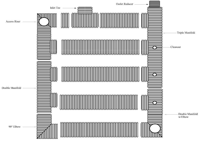
Typical Detention / Retention System Layout (Plan View)
